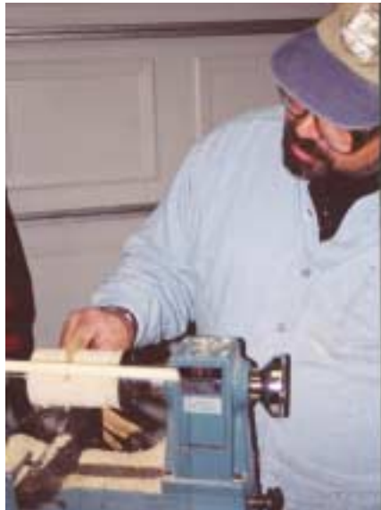
Cylinder turned to proper diameter
