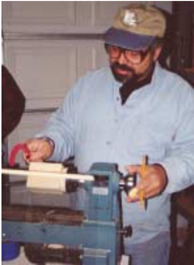
Steve Rome with his jig for marking and checking the shape of the sphere
