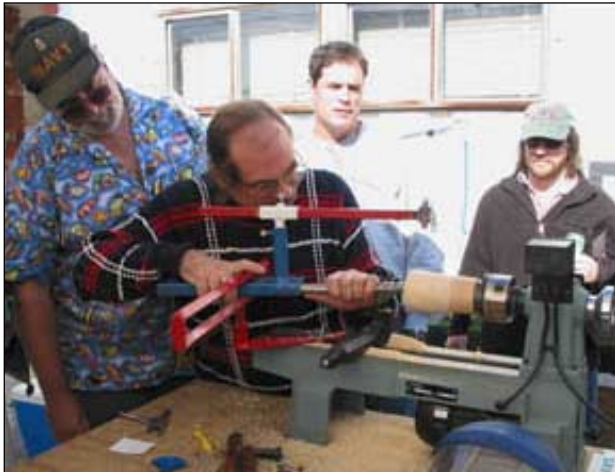
Club members, under O.B.'s watchful eye, try out his hollowing jig (above) and fluting setup (right)
