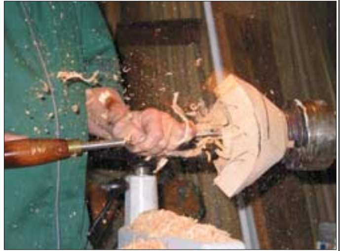
Hollowing out the inside of the bowl
