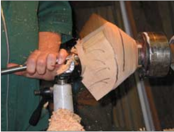
Hollowing out the inside of the bowl
