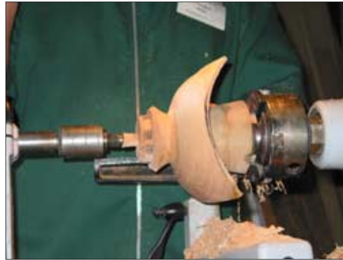
Form the base, sand and finish the outside using your finish of choice
