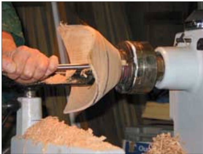
Hollowing out the inside of the bowl
