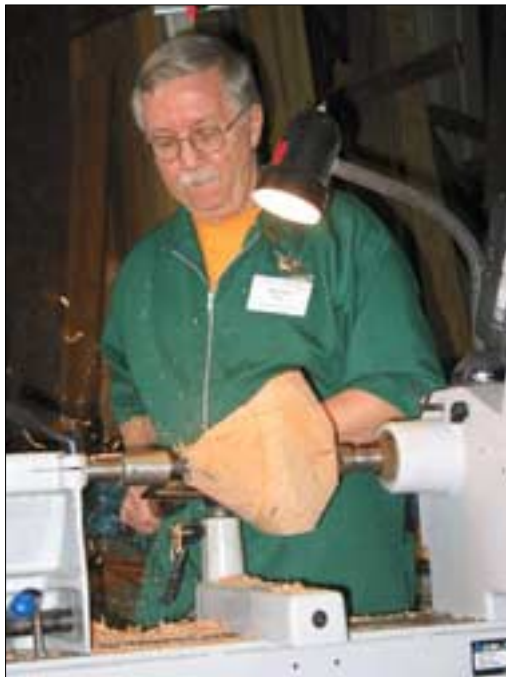
Forming a “cone shape” with base of cone at the live center
