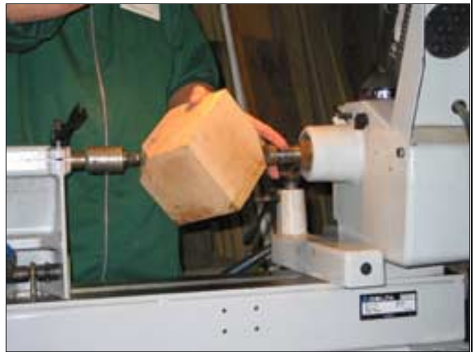
The Cube – For an Oil Confetti Lamp Hershel starts with a 6” cube. Remove opposite corners to mount on the lathe
