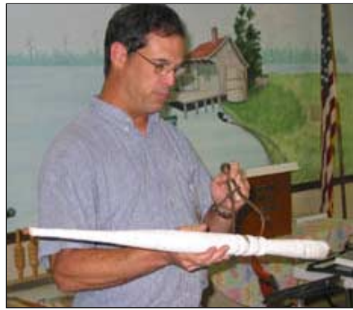
Using calipers, Paul measure the size of the bead he will duplicate on his spindle
