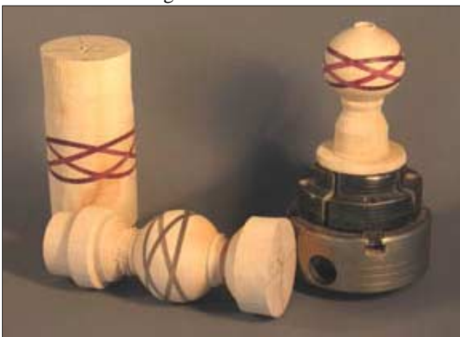
Shown are three ornaments in various stages of being turned into a ball.
