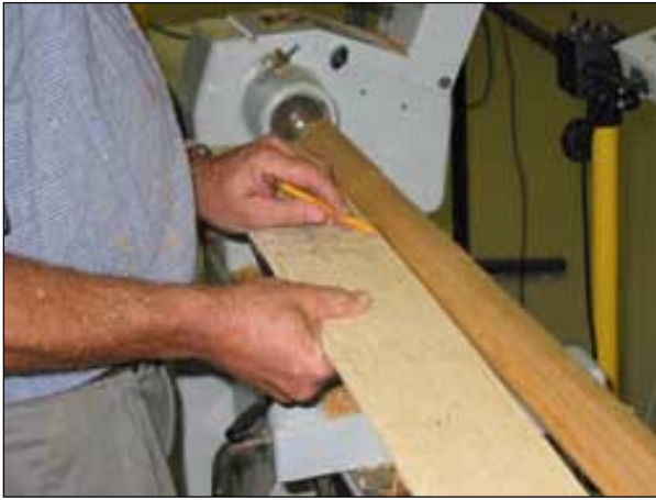
Paul transfers the locations of the various beads, coves, etc. from his template to the rounded out spindle.
