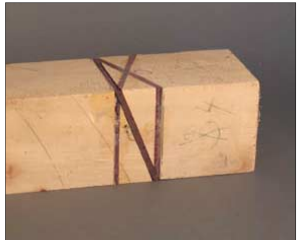
Glued up block with three crisscrossing bands of wood
