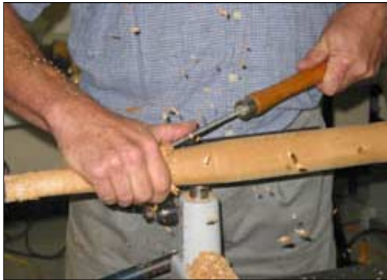
Paul transfers the locations of the various beads, coves, etc. from his template to the rounded out spindle.
