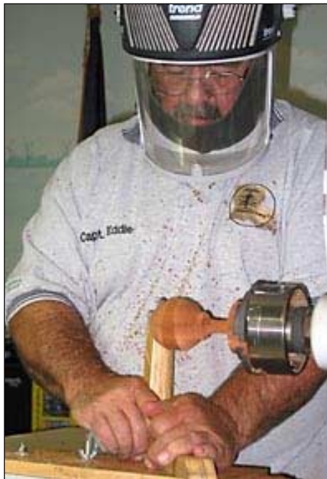
Eddie Castelin demonstrates how to cut a "ball" with a simple homemade jig.
