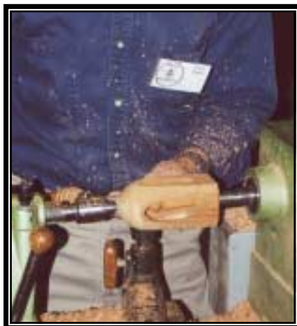
Turning the outside of the form
