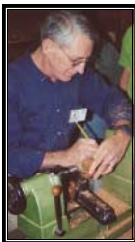
Marking the decorative inner spindle
