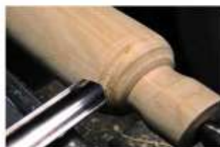
Catch with the side of the gouge
