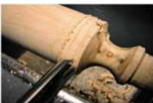
Catch with the nose of the gouge
