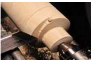
Catch with the toe of the skew
