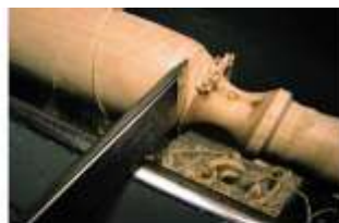
Catch with the heel of the skew
